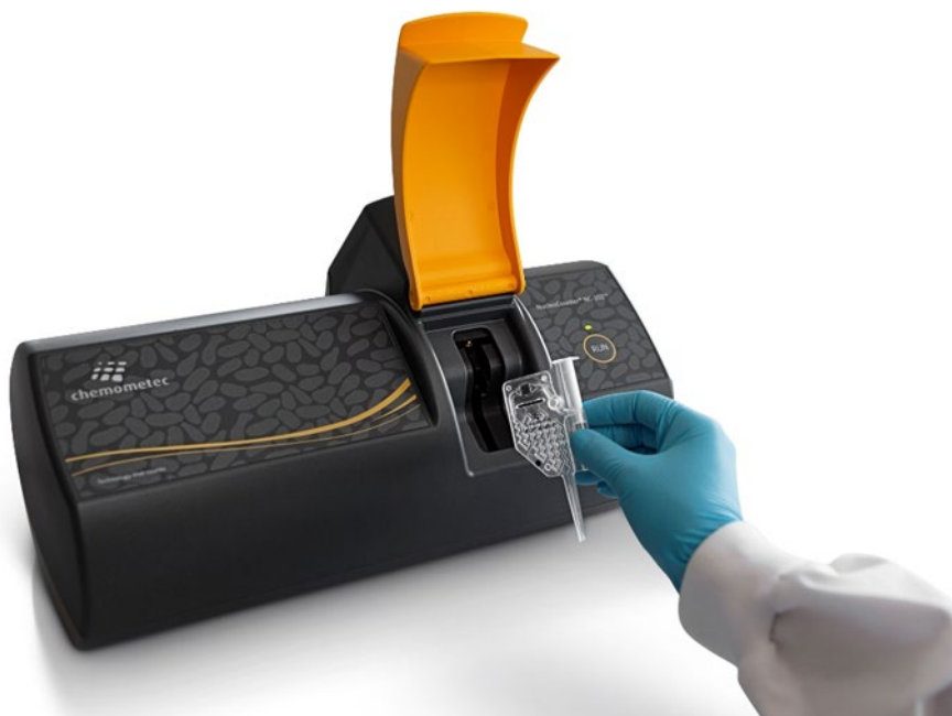
Figure 8: How to hold and place the Via2-Cassette™ in the fixture
