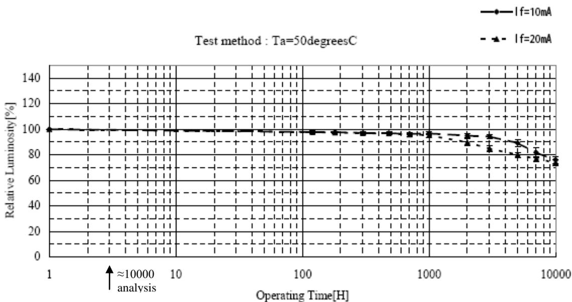
**Figure 1.** Relative Luminosity versus number of Operating hours for the Nichia LED NSPE500S at two different forward current conditions (data from Nichia Cooperation). The arrow indicates the aging of the LEDs corresponding to 10000 analyses made with the NucleoCounter<sup>®</sup>.
