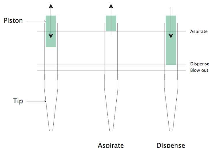
Figure 6 Illustration of the operation of a pipette
