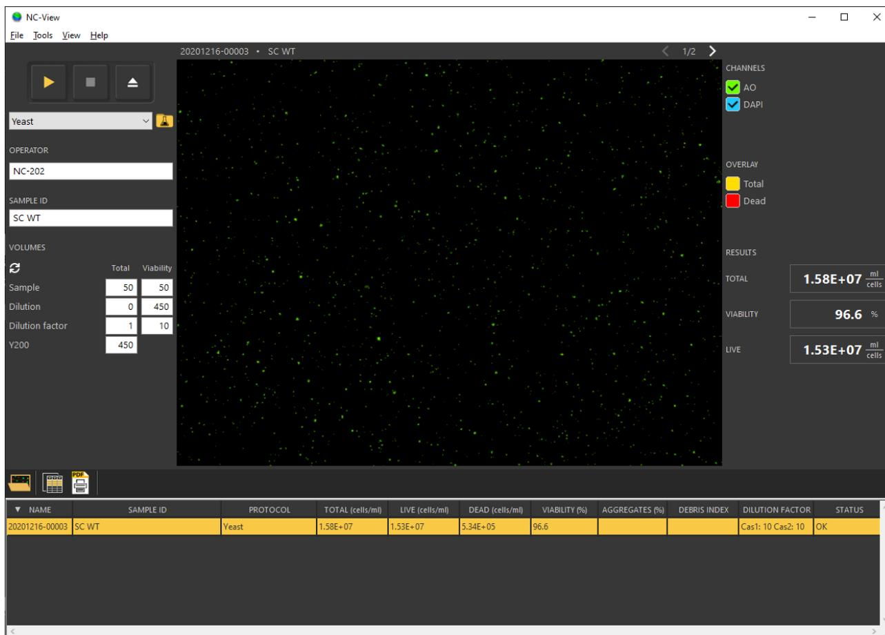
Picture of NC-View™ software after running a Yeast protocol on a *Saccharomyces cerevisiae* cell sample using the NucleoCounter® NC-202™. Acridine orange (AO) and DAPI channels are shown in green and blue, respectively. Enabling the image overlay displays total (yellow) and dead cells (red) identified by the software. Counting results are presented in the right panel and in the file list below.
