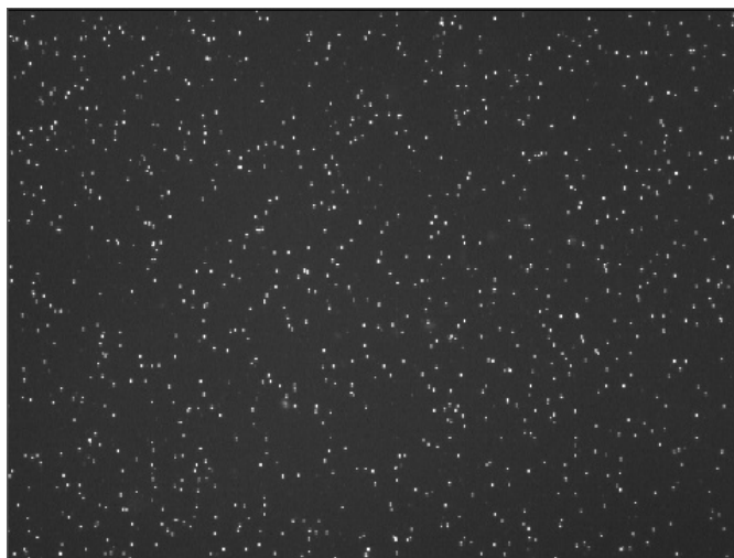
Image 1: Typical NucleoCounter ® image when viewed in NucleoView Software. Cells are shown as light dots. Cells have been treated with Reagent A100 and Reagent B before analysis in the NucleoCounter Instrument.
