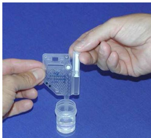
**Figure 3.** Loading the cassette with the lyzate mixture
