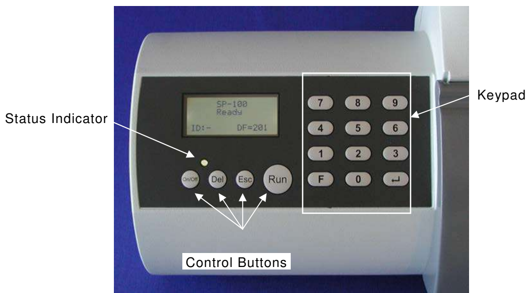
Figure 10. Control Buttons, Keypad and Status Indicator of NucleoCounter SP-100 instrument
