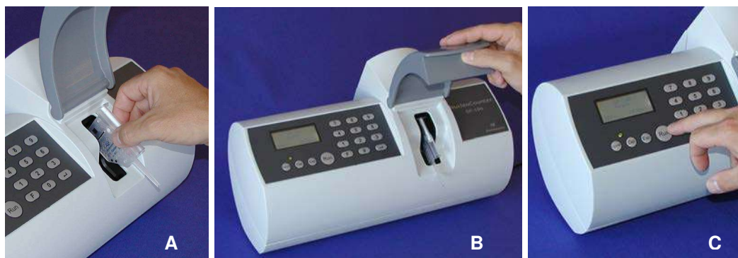
Figure 66. Insertion of cassette (A), closing the lid (B) and pressing the “Run” button (C)
