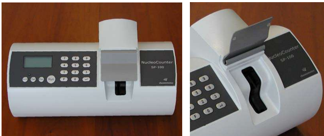
Figure 59. NucleoCounter SP-100 with the small version of the lid which can be used when many samples are being analyzed
