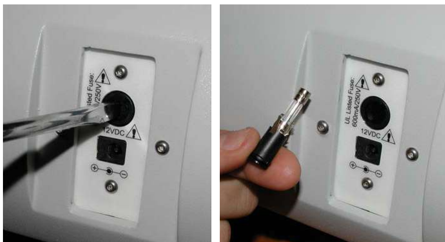
Figure 75. Location and removal of the fuse holder
