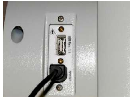
Figure 35 Connecting the Printer cable to the NucleoCounter (lower connector).
