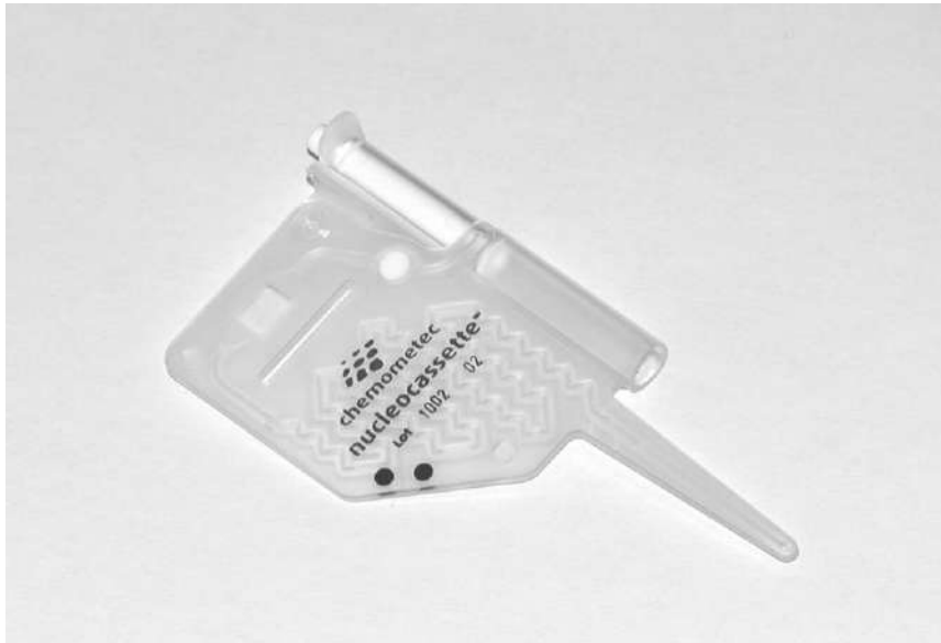
Figure 5 The NucleoCassette. The fluorescent dye, propidium iodide, is immobilized in the first part of the flow system.
