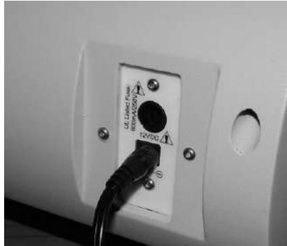
Figure 7. Connecting the 12VDC power cord plug to the NucleoCounter
