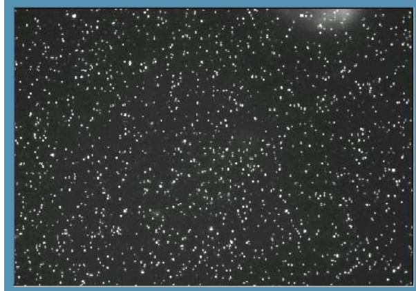
Figure 26. An image showing a contamination of the optical system, visible as a white cloudy phenomena in the upper right hand corner. If the contamination is stationary it should be removed using compressed air.
