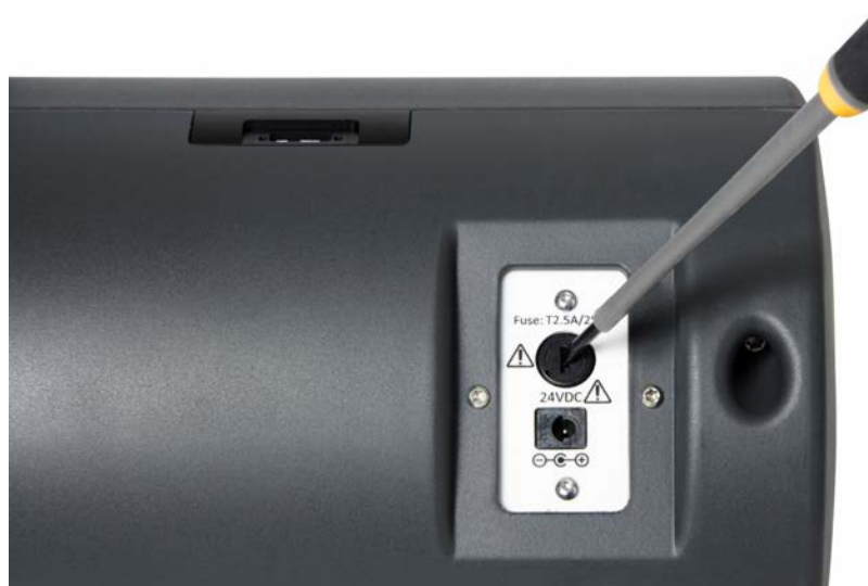
Figure 9: Location and removal of the fuse
