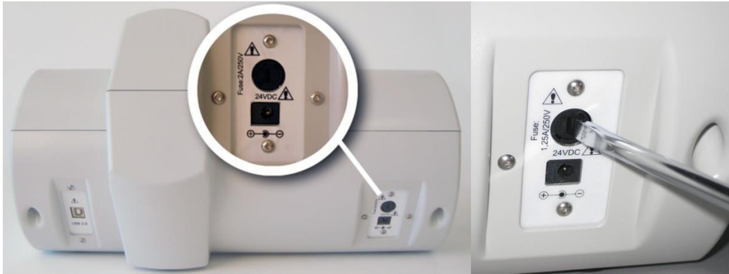
Figure 14. Location and removal of the fuse
