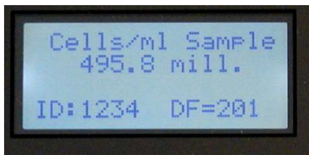
Figure 5. Result of the analysis shown in the LCD display (in this case the DF was 21).
