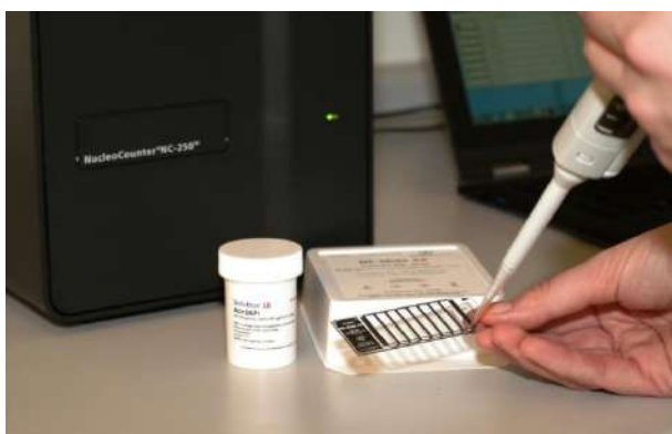
Figure 1: Viability and cell count assay with the NucleoCounter® NC-250™: (A) Mix cell sample with solution 18 and load the slide. Insert the slide in the instrument. (B) Press run and results are displayed continually for each chamber.
